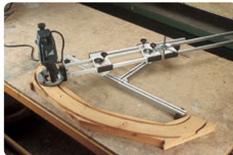
With the equipment “ELLIX” a perfect geometrical ellipse can be executed
