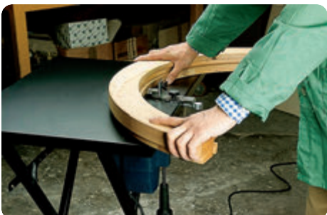
With the router table accessory and the ballbearing guide the execution of glazing bead is quick and easy.
