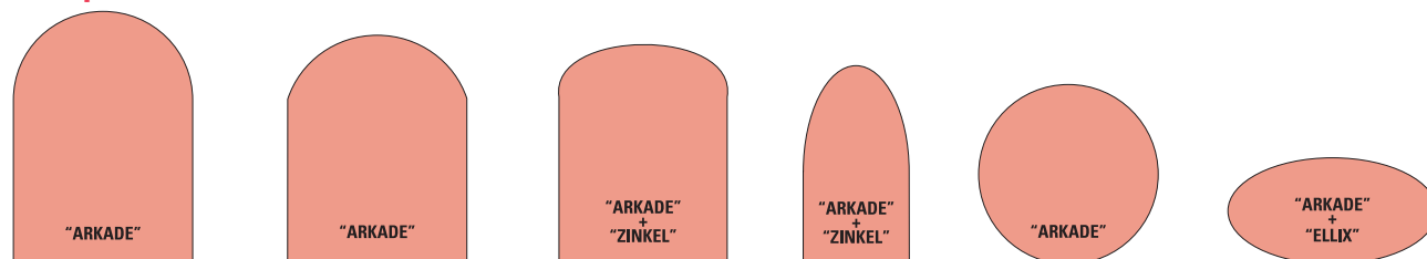
Item ELLISYSTEM “ELLISYSTEM” is the “last born” of our special equipments for producing arch frames. With “ELLISYSTEM” the customer can execute a perfect geometrical ellipse. Suitable for house restoration where the double radius arch is difficult to fit. Simple and easy to use, it keeps the same work procedure and features as “ARKADE” + “ELLIX”
