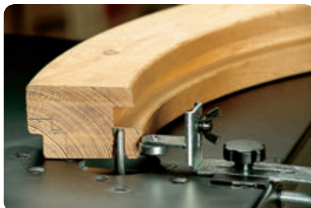
With the router table accessory and the ballbearing guide the execution of glazing bead is quick and easy.
